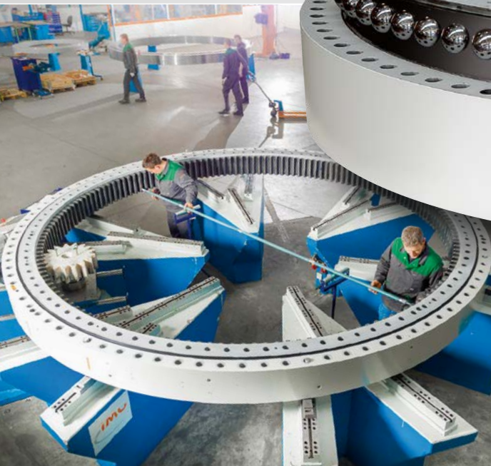
3 MW-class blade bearing, ► hydraulic pitch
