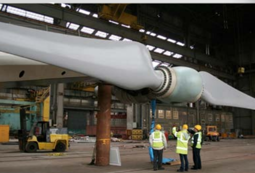
Blade Bearing for a 2 MW marine current turbine ▶
