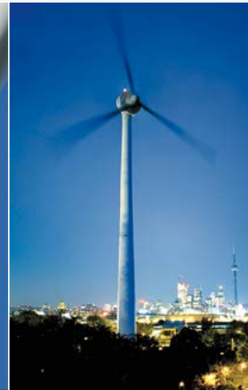
900 kW direct drive wind turbine generator
