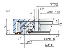
The mounting structure must support the housing to at least ø1091.
