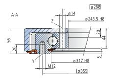
The mounting structure must support the housing to at least  $\emptyset 311$ .
