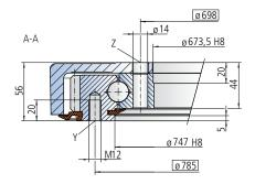
The mounting structure must support the housing to at least  $\emptyset 741$ .
