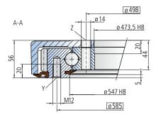
The mounting structure must support the housing to at least ø541.
