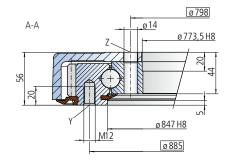
The mounting structure must support the housing to at least ø841.
