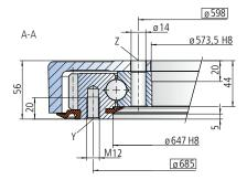
The mounting structure must support the housing to at least ø641.
