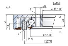
The mounting structure must support the housing to at least ø229.
