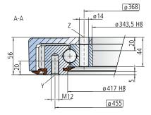
The mounting structure must support the housing to at least  $\emptyset 411$ .
